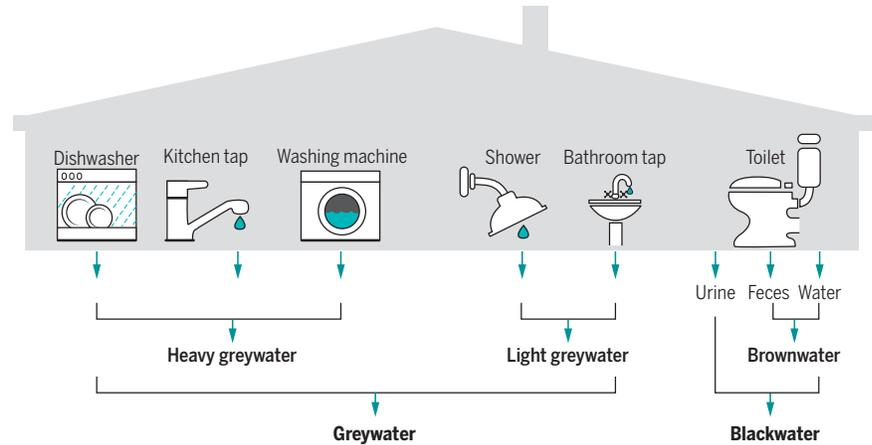
**Fig. 3. With source separation of wastewater in the household, new types of wastewater can be constructed for optimal treatment.** It is even possible to include treatment and recycling processes in a single device. This offers totally new perspectives for mass-produced, consumer-friendly wastewater treatment technology (for examples, see Table 2).
