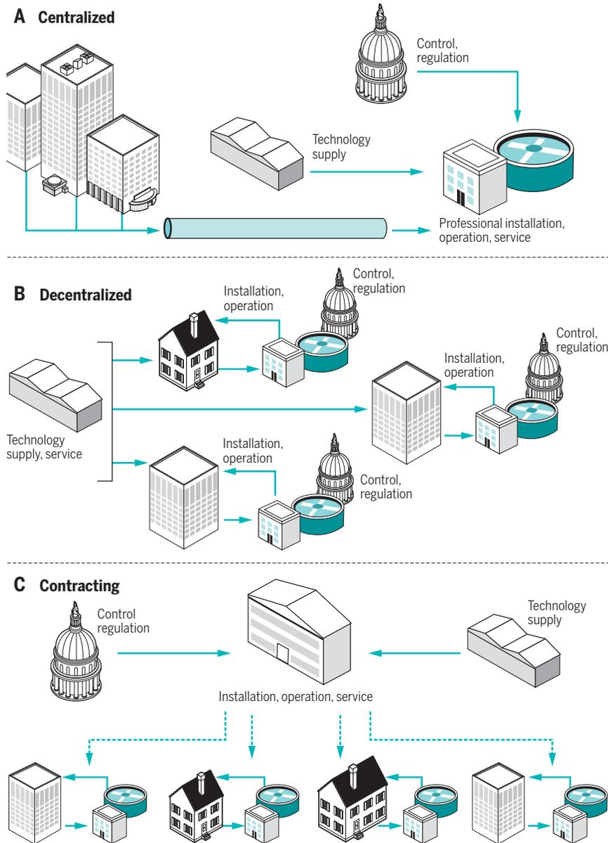
**Fig. 4. Alternatives for management of centralized and decentralized wastewater treatment plants.** (A) Fully centralized, (B) fully decentralized, and (C) contracting scheme for decentralized technology with centralized operation.
